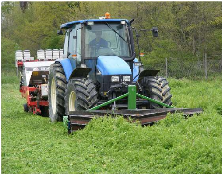
Fig. 1. Roller crimper (chevron design Rodale-type built by the farmer) mounted on the front of the tractor and coupled with a rear-mounted direct drill machine (Semeato SPE 06), carrying out hairy vetch (cv. Haymaker Plus) termination and sunflower (hybrid LG 55-57 HO) no-till sowing in one pass. Picture taken by Daniele Antichi at the farm hosting the trial (Tuscany, Italy) the 19th March 2014.
